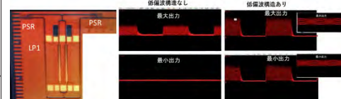
低偏波依存性シリコン細線pn接合型スイッチ (写真・時間波形) Low polarization dependent pn-junction-type silicon photonics switch (Photograph, time waveforms)
